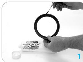
**Notice:** Gruvlok Xtreme Lubricant must be applied when used in dry pipe systems or freezer applications separation. Pipe joint separation may result in significant property damage and serious injury.
